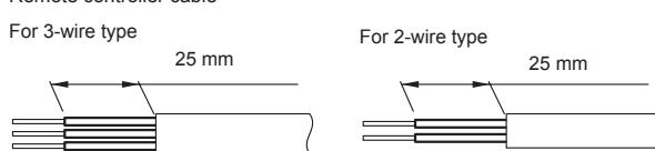
• Connect remote controller and transmission cables as shown in Fig. A.
